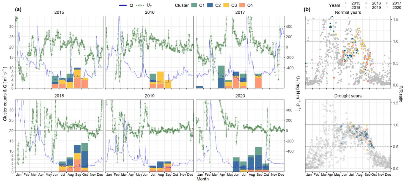
**Figure 4.3.** (a) Daily total retention rate  $U_T$  in each year based on the model-data fusion framework, and monthly counts of the four clusters of diel patterns. (b) Daily ratios of whole-stream gross primary production and respiration (i.e., P/R ratio) in the normal (2015-2017) and the drought (2018-2020) years. Note that, for subplot (b), P/R ratios on dates exhibiting diel patterns are highlighted with the same cluster colors as in subplot (a).
