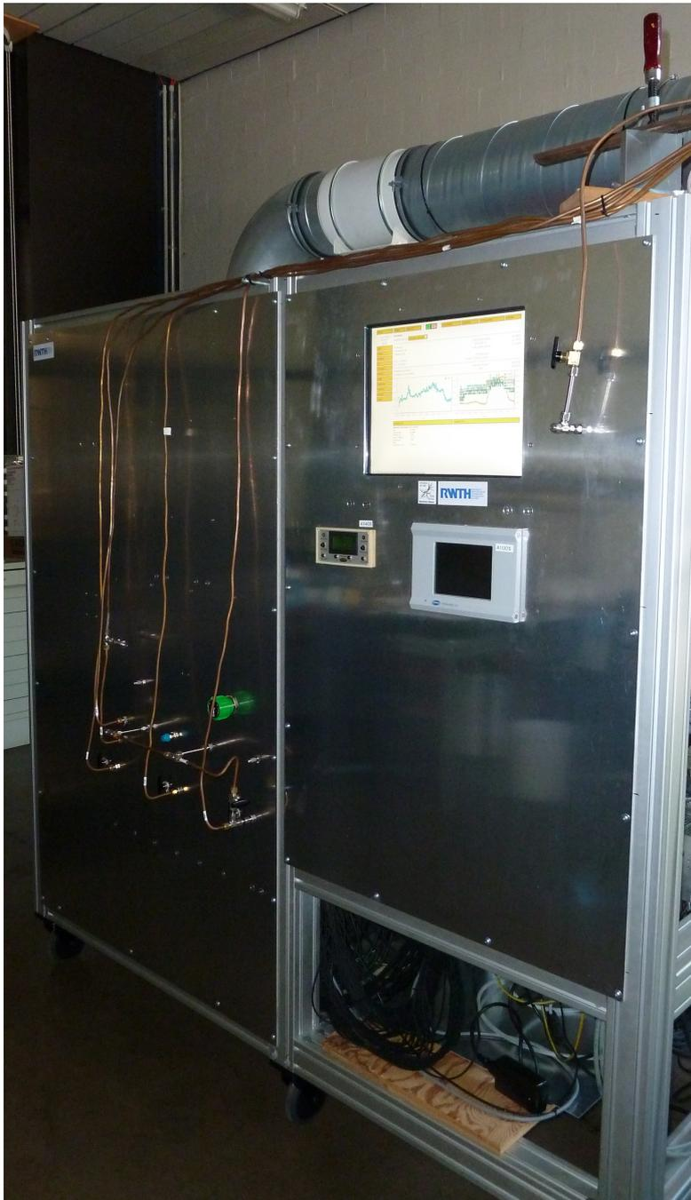
Figure 6.1.: Photo of the user interface of the UGMA. The touchscreen and the special readout modules for the  $\text{H}_2\text{O}$  and  $\text{O}_2$  sensor are shown on the right. On the left side the supply lines and the chamber are connected.
