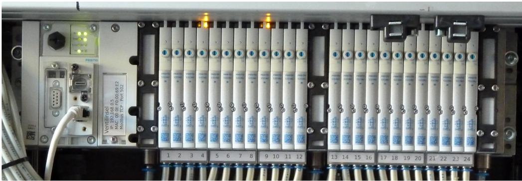
Figure 5.5.: Picture of the mounted valve island. On the bottom, the flexible tubing for the connection of the valve cylinders can be seen. The controller can be seen on the left side. The orange LEDs on the top indicate, which valves are currently switched on (valve 4 & 9).
