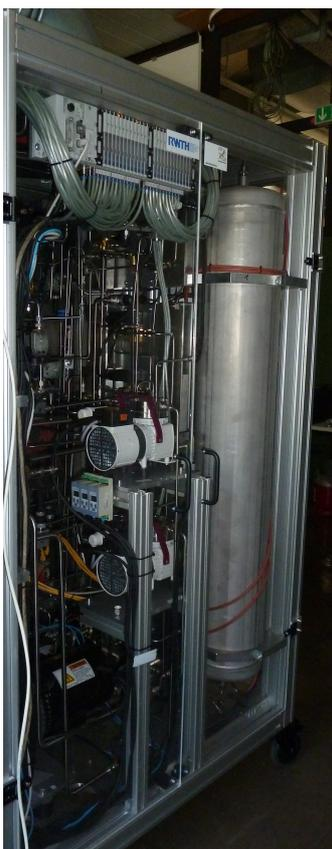
Figure 4.6.: View inside the gas handling section of the UGMA. On the right side one of the two buffer is shown. Directly in front of the buffer the pumps of the buffer loops are mounted. In the upper part one can see the valve island.
