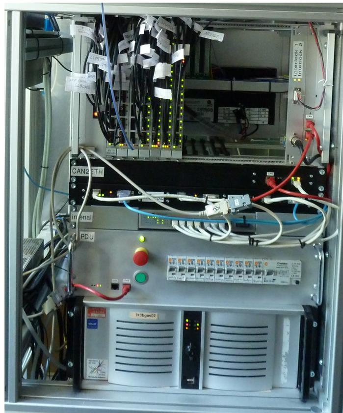
Figure 5.1.: Photo of the electronics readout. In the upper part the crate with the analogue and digital modules can be seen. Directly below this the CAN2ETH and the three RS232ETH modules are mounted. Above the PC, which is the lowest element the PDU and the internal Ethernet-switch is mounted. The white labels mark the cables which control the valves or are connected to the sensors.
