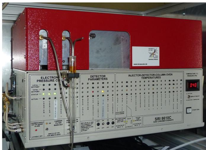
Figure 8.5.: Photo of the gas chromatograph.
