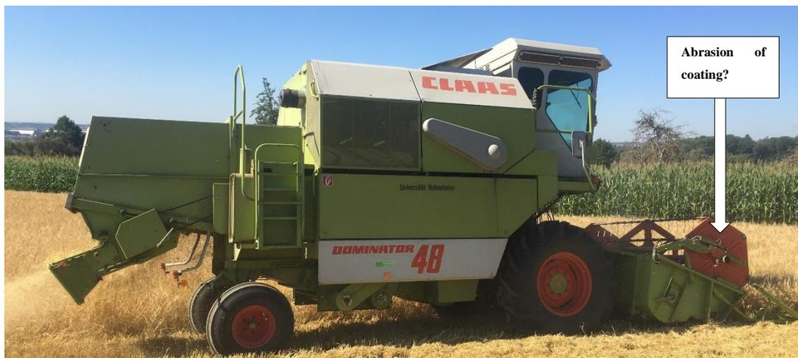
**Fig. S7-5.** Land machine harvesting summer barley on the site of the field experiment. Possible entry of red varnish particles due to abrasion of the red protective coating.
