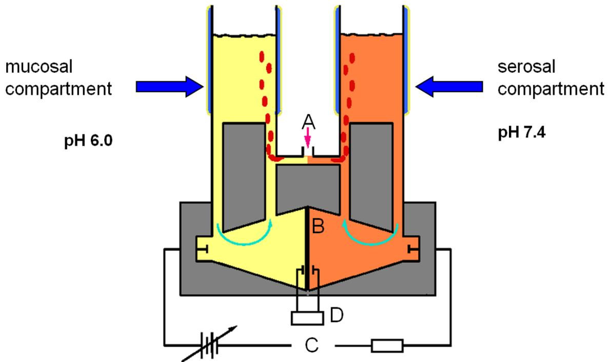
**Figure 7-1: Design of the Ussing type chamber: (A) gassing (95% O<sub>2</sub>, 5% CO<sub>2</sub>); (B) pig jejunal mucosa; (C) tissue conductance (Gt); (D) short-circuit current. Hanks' balanced salt solution at + 37°C was used as medium. Modified according to (Deußer, 2010).**
