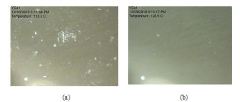
Fig. 8. Optical micrographs of CaSt, (1%) dispersed in mineral oil at a. 113 °C and b. 128 °C
